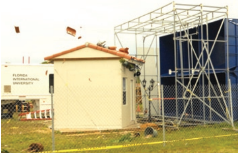
Clay roof tiles falling during testing
